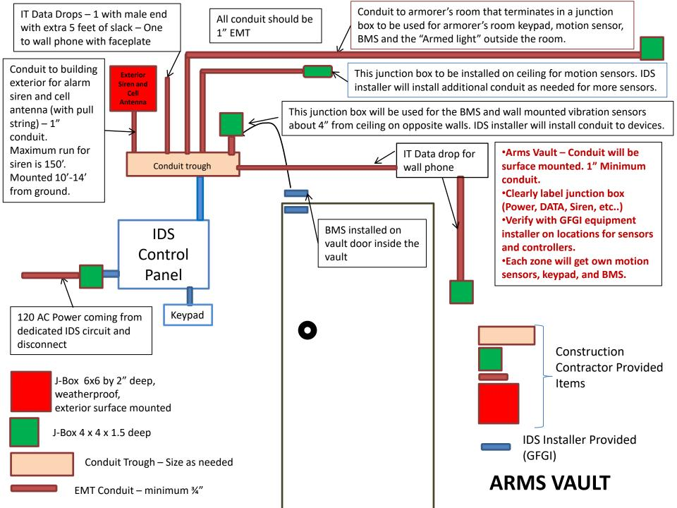
One IDS panel for both the Vault and Armorer's room. IDS panel will have one zone for Vault and one zone for Armorer's room.
